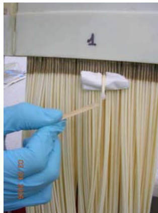
Figure 2. Application of epoxy
